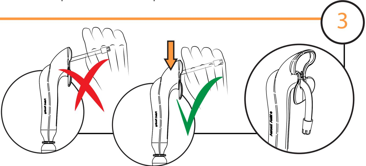
Tip: As you pull down, the saliva ejector should go beyond the pinching point and lock into position.
